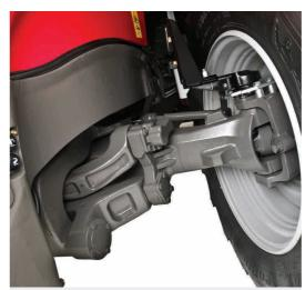
Massey Ferguson's 'QuadLink' suspended front axle further enhances ride comfort and control. It has a compact, simple design that automatically maintains a constant suspension height, regardless of axle load.
