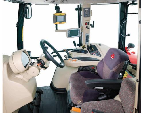
The Command Control Armrest can be specified with a multifunction joystick. When not required for use with a loader, for example, using the optional Datatronic 4, the buttons can be programmed to operate other functions including:
