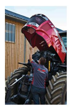
The single piece bonnet lifts fully to allow excellent access for full servicing
