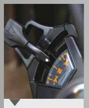
**MF Control Lever** The PowerShuttle is operated by the unique MF Power Control lever which also provides an additional control for travel direction changes, powershift changes and a declutch function for inching.
