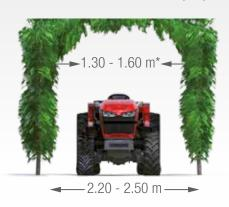
Low profile version ideal for work under trees, in polytunnels and in canopied vineyards. Suitable for row widths of 2.2-2.5m.
