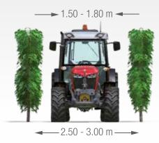
From 1.5m width, ideal for more extensive vineyards & fruit orchards with rows from 2.5 to 3.0m. A more substantial tractor with a wider front axle and a more spacious cab.
