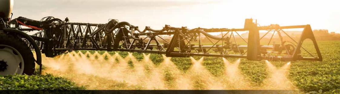
The booms are available in 28 or 30 meter widths with the following options fitted as standard to every machine:
