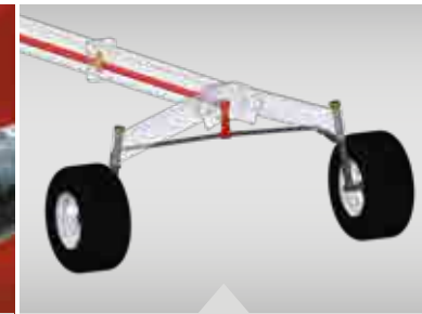
Track rods as already used in commercial vehicles
