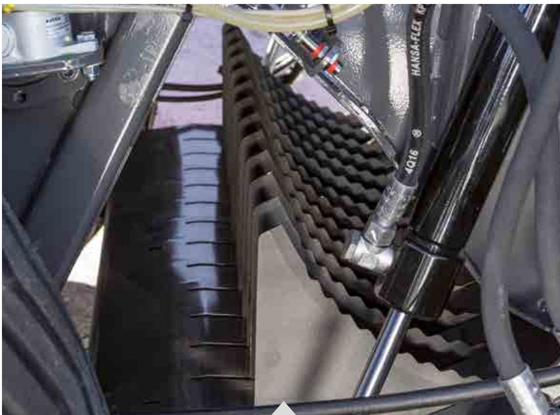
Xtracut 13 rotor features 90mm crop cutting length
