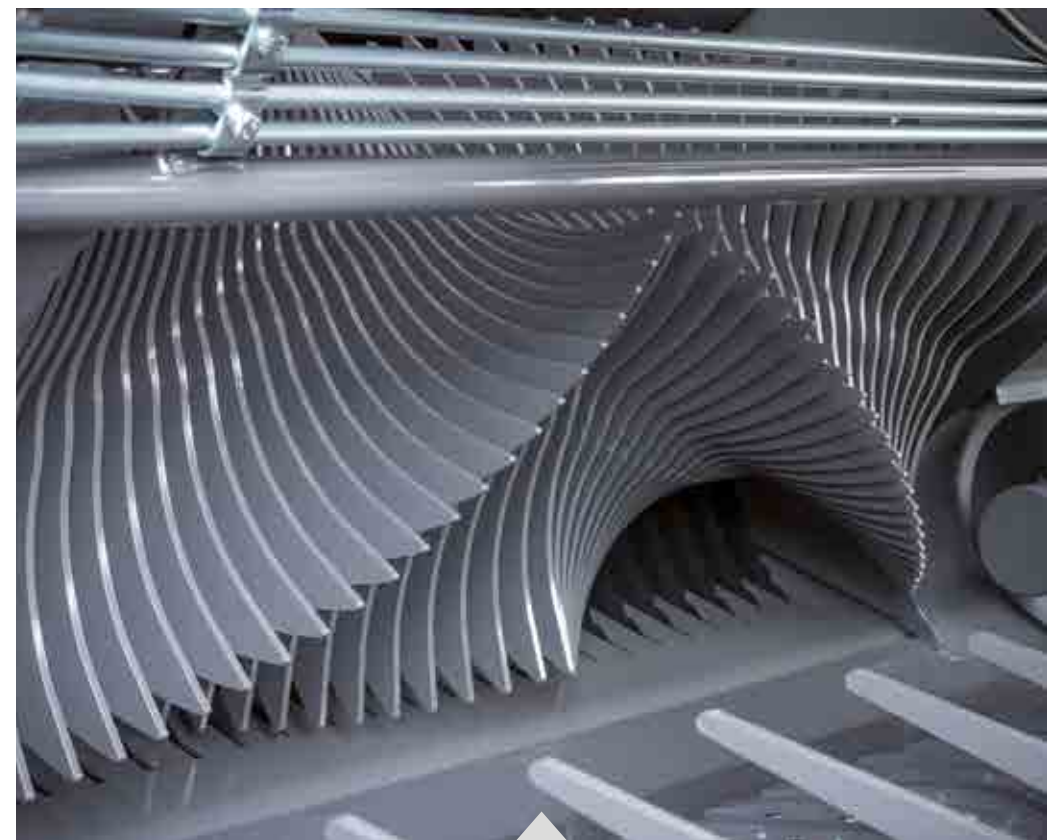
Xtracut 25 rotor has 4-tines design increasing chopping capacity
