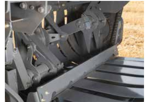
The Packer tines ensure even feed into the pre-compression chamber.
