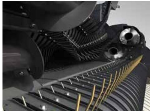
Cutter balers are also fitted with 'Quad' augers ensuring a consistent feed into the ProCut Rotor.
