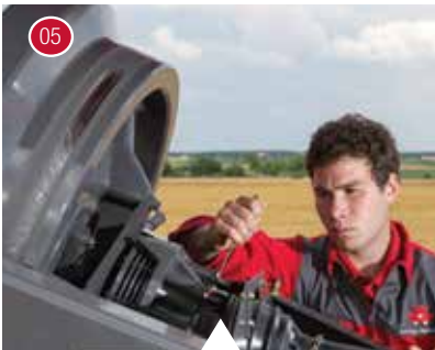
05 Adjusting the flywheel slip clutch.
