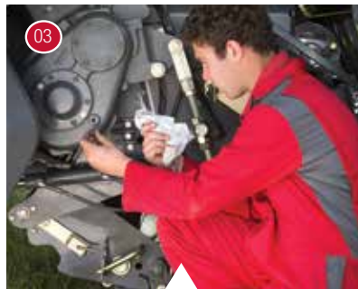
03 Checking the cutter gearbox oil level.
