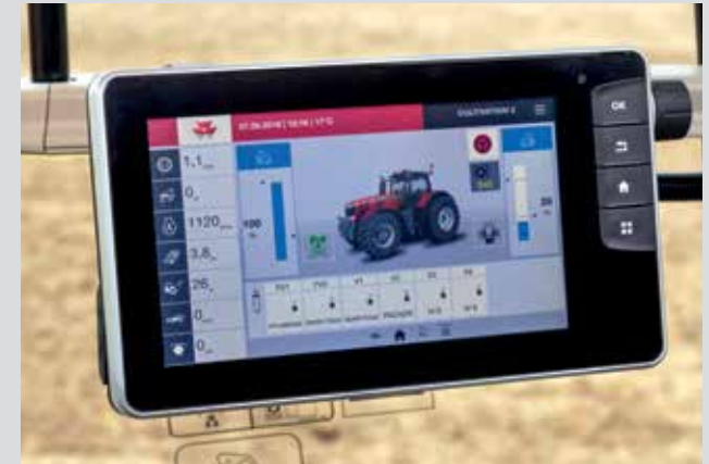
Controlling the baler via the tractor ISOBUS terminal.
