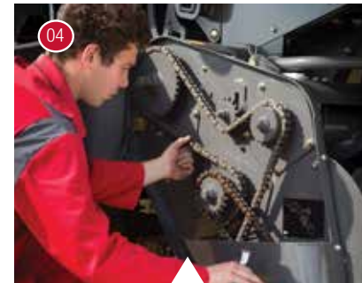
04 Checking the pick-up chain tensions.
