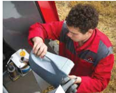
Refilling the automatic chain oiler.
