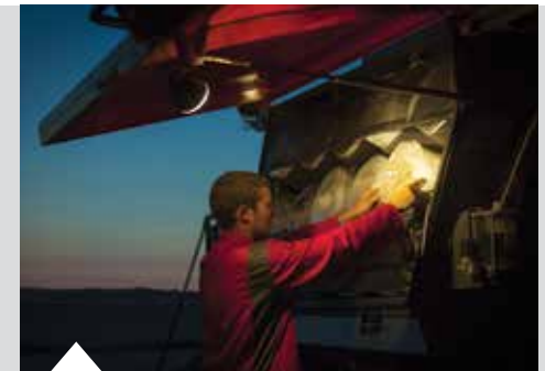
Twine box lighting allows easy night time refilling.
