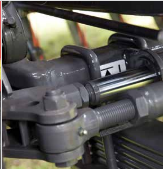
Rear axle hydraulic steering lock.
