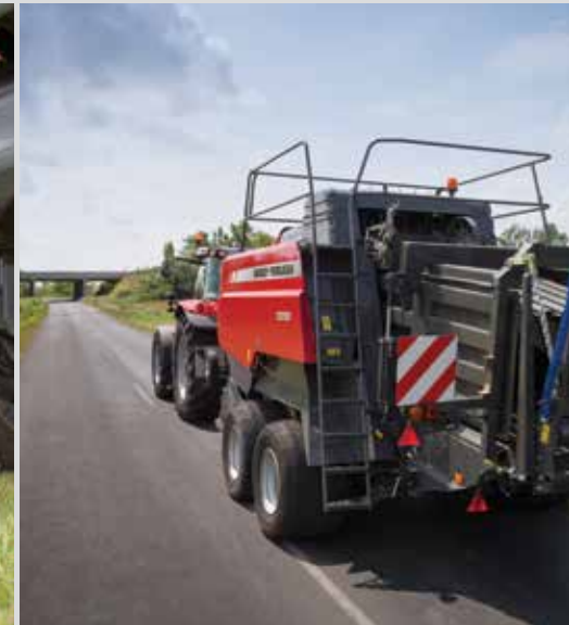
The tandem axle allows for high road speed and gives superb ride comfort between fields.
