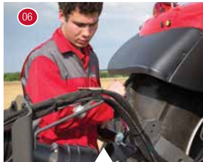
06 Greasing the PTO shaft.
