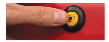
A REAR-MOUNTED STATIONARY PTO SWITCH MAKES IT EASY to engage and disengage the PTO from the rear of the tractor — a very
