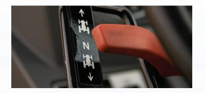
A HANDY SHUTTLE-SHIFT LEVER — Lets you change direction fast and easy — ideal for loader work, and located on the steering column.
