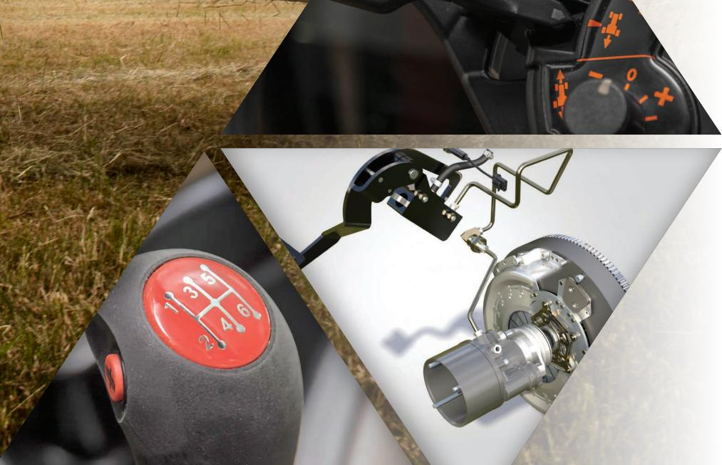
**POWER CONTROL LEVER** — The left-hand Power Control lever provides convenient and simple three-in-one operation through the state-of-the-art transmission. Operators can shuttle between forward and reverse without clutching, making jobs that require frequent direction changes, like loader work, a breeze. Shuttle responsiveness can be modified by simply adjusting the comfort control dial.
