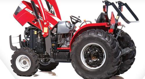
**THE STANDARD FOLDING ROPS** allow an MF E Series to fit beneath a standard 7-foot garage door.
