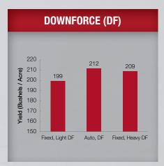
Payback: When not using DeltaForce and planting with fixed downforce pressure that was too low, the average loss was 6.3% per acre. When planting with fixed downforce pressure that was too high, the average loss was 1.4% per acre.
