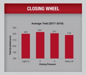
Payback: When closing wheels were in setting 2 compared to setting 4, we saw an increase of 2.3% in our return per acre.
