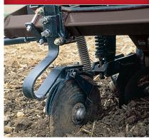
Designed for conventional and minimum-till applications. Two 13.5 in. (343 mm) diameter discs are C-spring mounted to an adjustable clamp.
