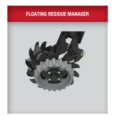
13 in. (330 mm) SharkTooth or finger wheels and depth bands provide aggressive residue movement from the path of the row unit. The unit-mounted residue wheels float over the surface, and the depth bands assure the right depth of operation.
