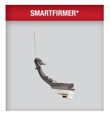
Precision Planting's SmartFirmer® is a seed-firmer sensor that measures the seed environment while firming each seed into the bottom of the trench. SmartFirmer helps you know that the seed is placed into a good environment and determines what type of variability you may have in your field according to different metrics, including moisture, temperature, uniformity, residue and organic matter.
