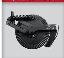
Designed for no-till planting conditions, this 17 in. (432 mm) disc and knife work well in firm, no-till soil that has residue on the soil surface. The disc cuts residue at the soil surface, and the trailing knife places the fertilizer with minimum soil disturbance.
