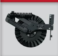
Designed for no-till, minimum-till and conventional tillage operations, this single disc fertilizer opener/ liquid injector features a spring-mounted tine injector nozzle for liquid fertilizer application. Liquid fertilizer is placed in the soil without the use of a knife, providing plug-free operation.
