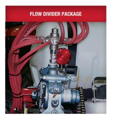
The piston pump flow divider provides optimum liquid fertilizer metering accuracy to each fertilizer opener. The application rate per acre remains constant over a wide range of planting speeds.
