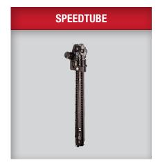
SpeedTube<sup>TM</sup> works with other systems from Precision Planting to create a high-speed planting system that ensures that as you speed up, yield potential is not going down. SpeedTube uses a flighted belt to control the decent of the seeds into the seed trench, and they don't tumble in the furrow because the seed release is matched to ground speed.
