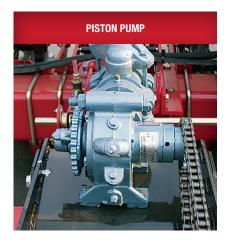
The variable-stroke, double-acting, single- or doublepiston metering pump dispenses a consistent flow of liquid fertilizer. All internal parts that come in contact with the fertilizer are stainless steel.
