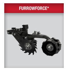
FurrowForce® from Precision Planting is an automated row-by-row control system that provides visibility to closing performance on the 20l20 display in the cab. FurrowForce uses two stages to both close the furrow and manage soil density. The first stage pinch wheels are set wider than traditional systems and move soil horizontally to remove air gaps. Following are the second-stage stitch wheels that create the proper soil density for moisture retention and optimal germination.
