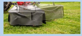
**MECHANICAL ANTI-COLLISION** — A breakaway system allows for one or both wings to swing back and slightly up if struck with an immovable object
