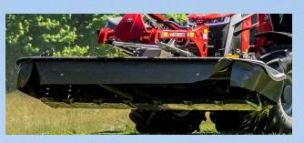
**RAZOREDGE CUTTER BAR** — The rugged and dependable one-piece welded cutter bar has been fitted into the 8612 and the 9614. Mow through the toughest crops with ease.
