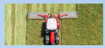
**TWO WORKING POSITION WIDTHS** — The mower support arms now have two bolted positions for the mowers to mount. The 8612 can adjust from 27 feet, 4 inches to 28 feet, 4 inches, and the 9614 can adjust from 30 feet, 6 inches to 31 feet, 6 inches.
