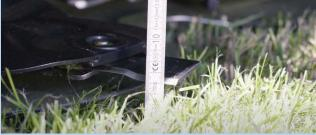
**STEPLESS CUTTING HEIGHT** — Cutting height can be seamlessly adjusted from 1.6 inches to 2.75 inches for all your crops and conditions.
