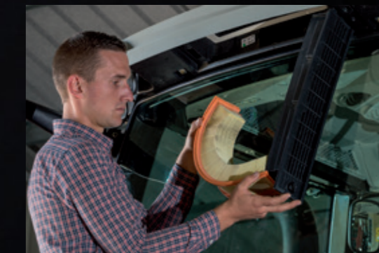
The cab air filter can be removed easily for cleaning.
