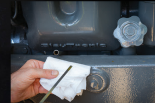
The waisted bonnet and front axle design ensures comfortable access to the engine oil filters and oil dipstick.
