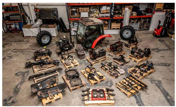
What does it take to refurbish an 18-year-old Massey Ferguson 5455 which has done more than 18,000 hours of hard labour and transform it back to factory condition? Well, more than 100 hours of diagnosis and in excess of 1100 genuine AGCO parts – all of which come with a full 12 month warranty - for a start...
