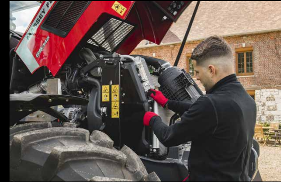
Cooling package is easily accessible to make cleaning faster and easier.
