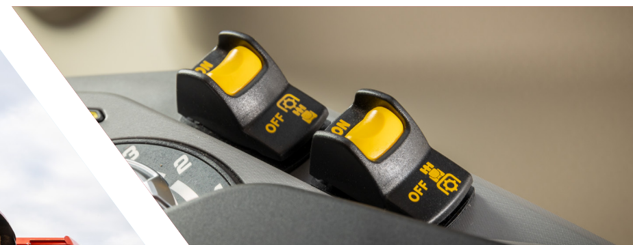
Electro-hydraulic PTO speed selection
