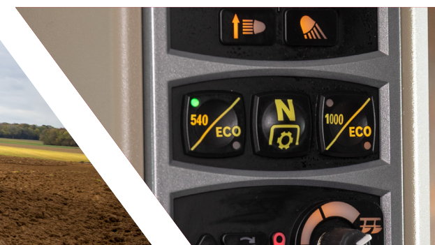
Electro-hydraulic PTO speed selection
