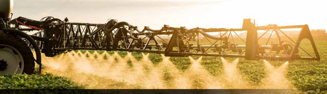
The booms are available in 28 or 30 meter widths with the following options fitted as standard to every machine:
