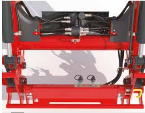
Cross-tube houses hydraulic components and provides strength without impacting the visibility
