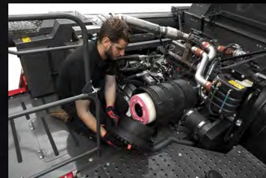
Checking and cleaning the air filter
