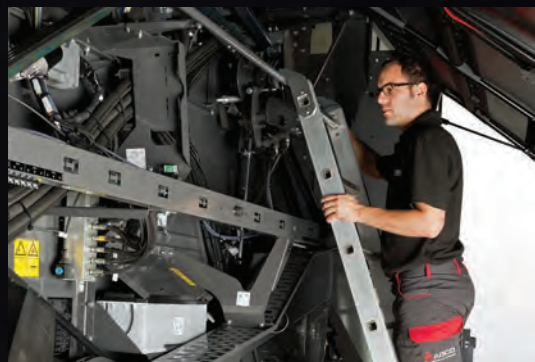
Ladder rail makes inspection easy and safe
