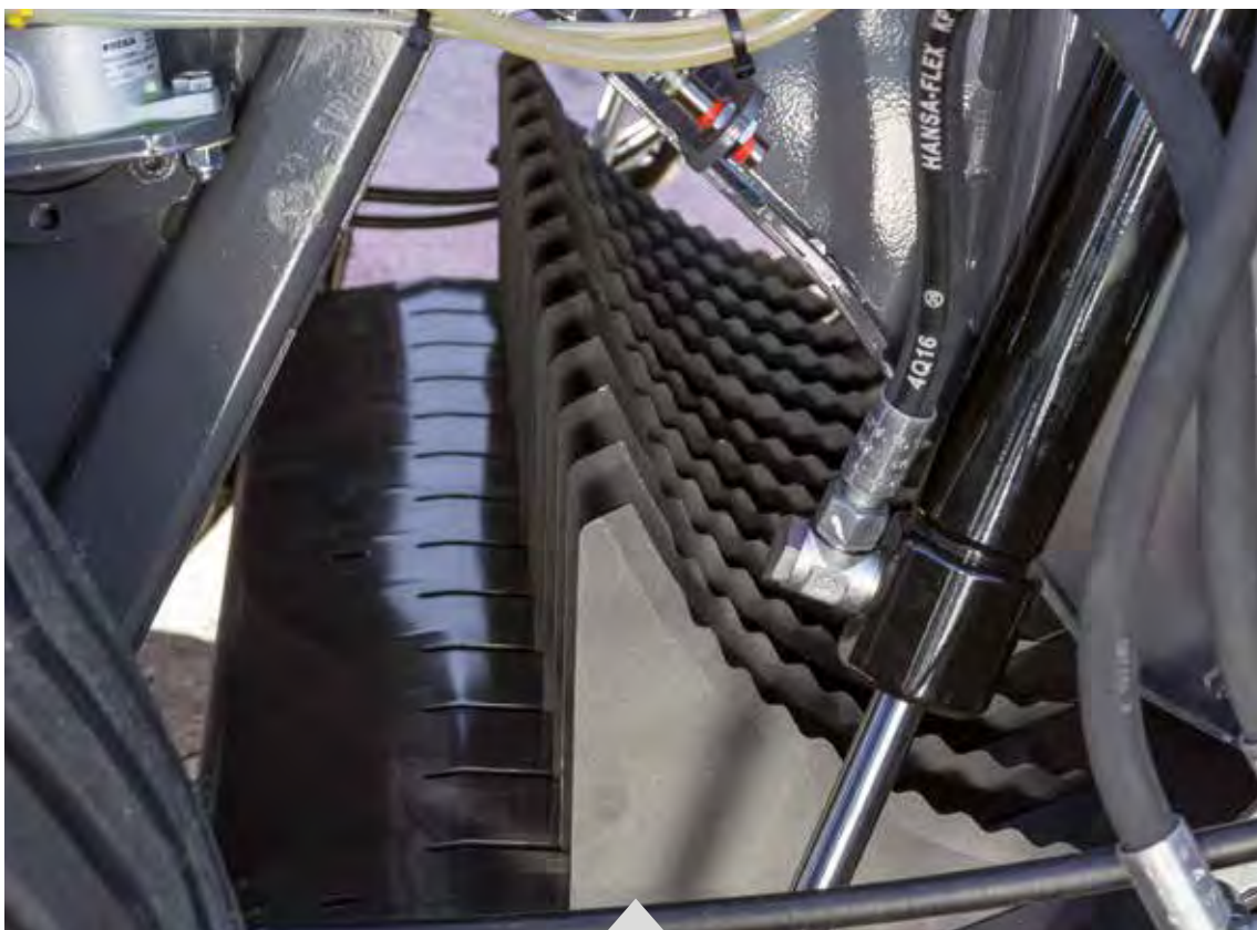
Xtracut 13 rotor features 90mm crop cutting length
