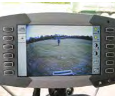
A video camera can be easily added to your pre-wired baler. The C1000 Baler Monitor is full colour video compatible as standard.
