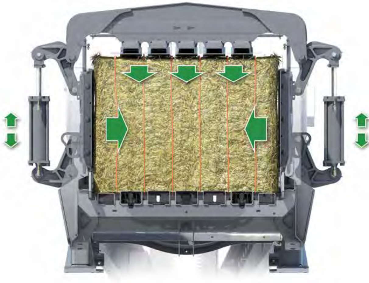
Three way double acting density system.
