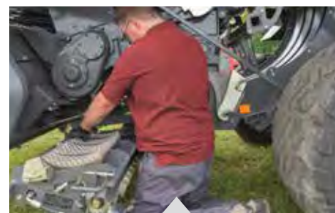
Ample accessibility offering straightforward knife removal
