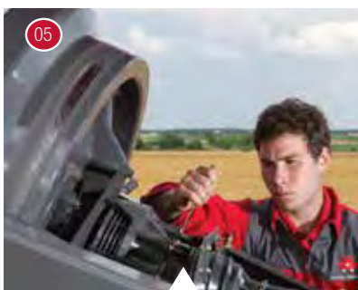
05 Adjusting the flywheel slip clutch.
