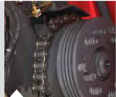
Automatic Chain Lubrication across the full width of the chain.
