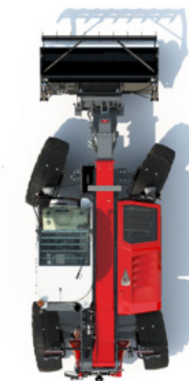
SEMI CRAB-STEER mode - set rear wheel angle - useful for applications such as silage or barn cleaning.
