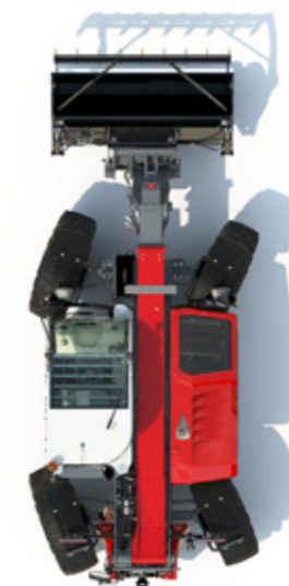
FOUR-WHEEL steering mode - for minimum turning circles.
