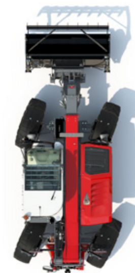
CRAB-STEER mode - for efficient filling and grading and working alongside walls in confined spaces.
