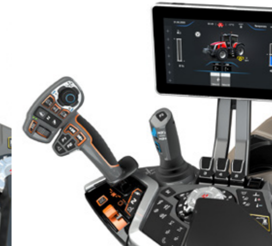
The MF Exclusive cab option with MultiPad control lever and electronic joystick.
