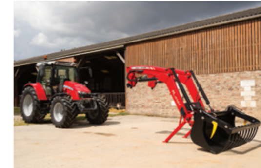
▲ STEP 1. Simply drive the tractor into the parked loader. The loader will smoothly meet with the loader subframe.
