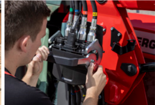
▲ STEP 2. The optional quick coupler speeds loader, hydraulic connection while avoiding oil spillage.
