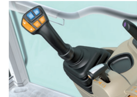
Essential cab option with mechanical multifunction joystick.
