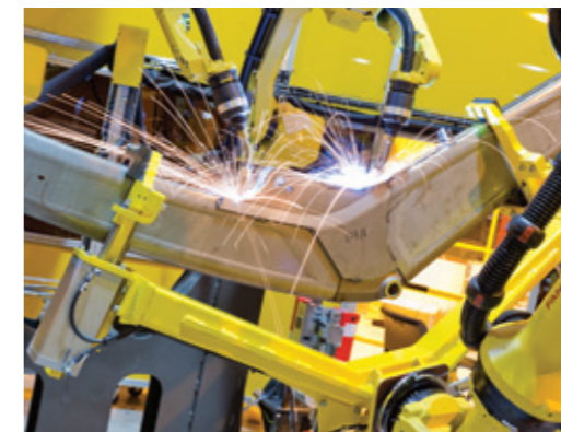
▲ Robotised welding ensures accuracy and strength.
