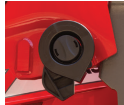
▲ STEP 3. By operating the lift cylinder, the semi-automatic 'Lock and Go' system speeds and simplifies loader hook up.
