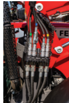
▲ Base configuration with flat face single couplers
