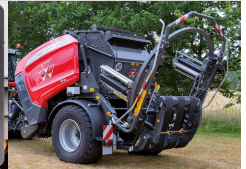
The wrapper unit can be folded up for safe and convenient field to field transport
