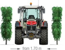
From 1.70 m wide, ideal for hillside vineyards Available with a low profile or flat-floor cab, this versatile tractor is designed and built for hilly terrain. Also the perfect light utility
