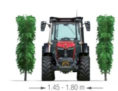
From 1.45 m wide and ideal for more extensive vineyards and fruit orchards, the MF 3FR is a more substantial tractor with a wider front axle and a more spacious cab. available from 75 hp to 120 hp. It is also available in a platform version up to 105 hp.
