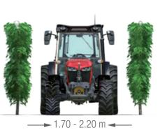
or orchards with a wider front and rear axle. Fitted with a more spacious cab, it delivers power from 75 to 120 hp. The MF 3WF is also tractor, the MF 3AL offers power from 75 hp available in a platform version up to 105 hp. to 105 hp.
