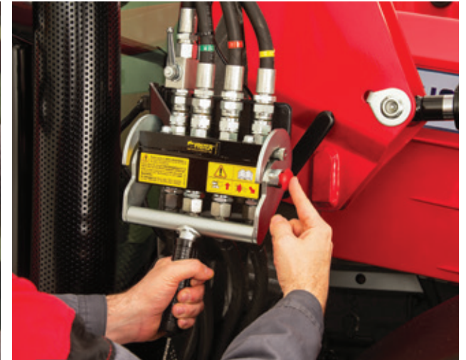
Disconnect the hydraulic and electrical connections
