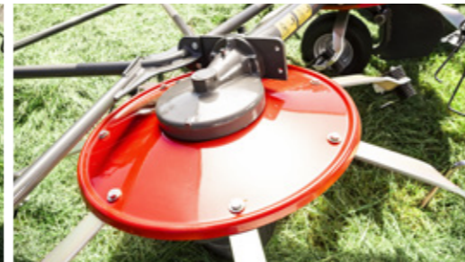
Large rotor provides you with high crop capacity at a low rotor speed.
