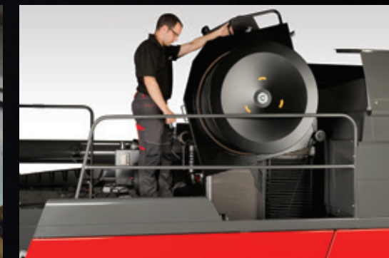
Safe and simple access for radiator cleaning
