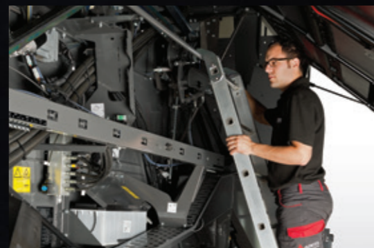
Ladder rail makes inspection easy and safe
