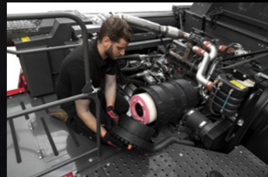
Checking and cleaning the air filter
