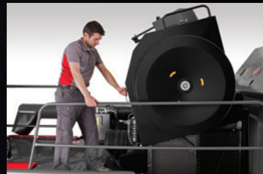
Safe and simple access for radiator cleaning
