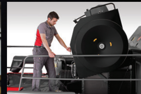
Safe and simple access for radiator cleaning
