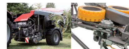
Twelve film roll holders are conveniently located at a comfortable height on both sides of the baler and with two additional rolls installed on the wrapper, increasing uptime in the field.
