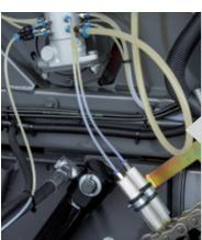
Automatic chain lubrication with individual adjustment for each chain guarantees sufficient oil supply, reduces maintenance time and extends chain service life. For added durability the highest quality chains are used throughout
