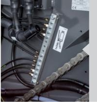
Regular and sufficient lubrication of roller bearings is extremely important, particularly in adverse conditions, for example when baling silage. Centralized grease banks for roller bearing lubrication are located in convenient positions for easier access and reduced service time.
