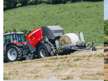
Once the bale is transferred to the centre of the wrapper table, a hydraulically driven wrapper ring begins its rotation even before the tailgate is fully closed, completing the cycle well before the next bale is formed. Designed to withstand the heaviest bale loads, the robust frame with its quiet running gear operates at up to 35 rpm smoothly for trouble free wrapping, bale after bale.
