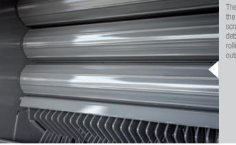
The roller support bearings in the bale chamber feature new scrapers, efficiently removing debris and moisture from the roller bearings and keeping the outside panels clean.
