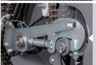
The simple, fast and efficient mechanical tail-gate locking device is now enhanced with pressure sensors on both sides and features left-right indication allowing the operator to monitor the outer layers of bale.
