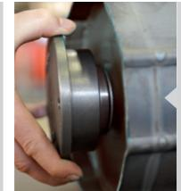
The bale chamber can experience extreme loads with forces from all directions. The clever bearing housing design allows some movement of the rollers to eliminate major axial loads occurring during
