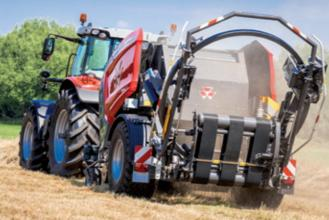
In transport mode the wrapper ring is folded forwards, reducing the overall machine length to just 5.9 m for safer transport and improved manoeuvrability.
