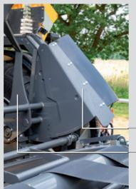
In addition to the transfer arm, the design features two active guiding plates on both sides of the baler clearly directing the bale to the centre of the wrapper plate allowing for a faster and more secure transfer cycle. For added safety in hillside conditions the unique slope transfer mode allows for the transfer arm to move more slowly while the wrapper ring is lifted higher to receive the bale. This ensures that the bale will be securely delivered to the wrapper even in
