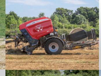
To ensure gentle bale unloading, the wrapping table is lowered, thus minimising the bale's rolling speed, preventing film damage and maintaining the ideal bale shape. An optional bale tipper puts bales on their ends, preventing them from rolling away and making for easier loading on the trailer. The operator can also choose between automatic and manual unloading modes.
