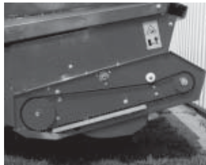
Below: Two speed gathering units with 2 sets of spring loaded chains per unit. Note high speed knife at the end of the gathering unit
