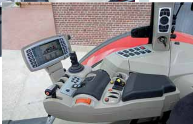
The armrest with Datatronic CCD looks after a large number of functions. Certain elements of the ergonomics within the cabin could do with improving, but overall the accommodation still notches a '++' in our test sheet (p18).
